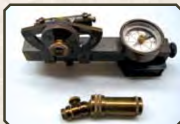
K&E Abney Level with Compass and Pentaprism, 1921. Catalog describes the Abney as having sufficient accuracy for military reconnaissance and preliminary surveys. The PentaPrism Range Finder is used to obtain distances. Cost $34.
